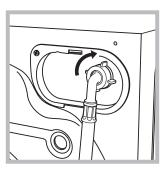
2. Connect the other end of the water inlet hose to the washerdryer, screwing it onto the appliance's cold water inlet, situated on the top right-hand side on the rear of the appliance (see figure).
