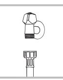
1. Connect the supply pipe by screwing it to a cold water tap using a 3/4 gas threaded connection (*see figure*). Before performing the connection, allow the water to run freely until it is perfectly clear.
